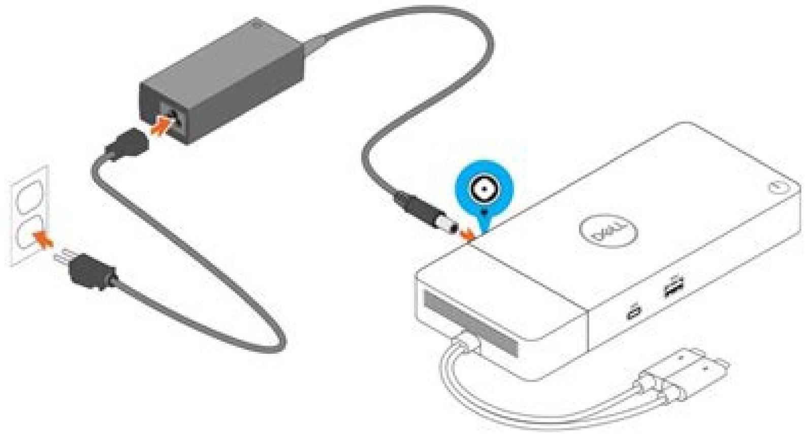
Figure 6. Connecting the AC Adapter
